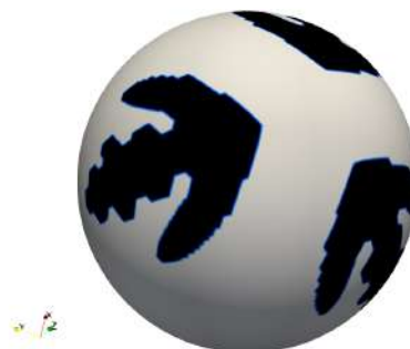
FIGURE 19. An experiment with three initial seeds. Each crystal grows symmetrically to the others.
